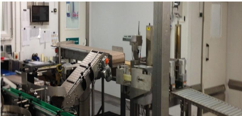
Line three appeared far more straightforward as there are only larger tubs, 1lb and 2lb, on this line which are boxed. The difficulties with line three were caused by a lack of space and the need for 1lb tubs to be diverted on to an existing conveyor when these were sleeved. All the tubs on line three are date coded and Codeology installed a short conveyor, after the existing metal checker, to serve as
